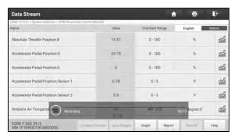
Tap • to end recording and save it. The saved file follows the naming rule: It begins with vehicle type, and then the product S/N and ends with record starting time (To differentiate between files, please configure the accurate system time).
