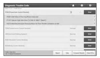
The tested system with fault code appears in red and the system with OK displays in green (normally).
