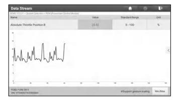
Min/Max: Tap to define the maximum / minimum value. Once the value goes beyond the specified value, the system will alarm.
