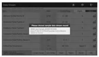
All the values you customized and saved in process of DS sampling will be imported into the **Standard Range** (See below) column for your comparison.
