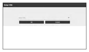
Input the VIN, and tap **OK**, the tablet will automatically identify the vehicle model and directly navigate to the diagnostic function selection menu.
